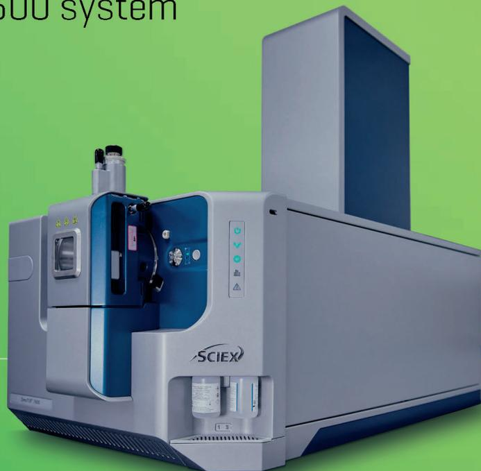
This high-resolution accurate mass system encompasses the power of the Zeno trap with electron activated dissociation (EAD) or Collision Induced Dissociation (CID) technologies, allowing you to uncover structural information that was previously inaccessible.
